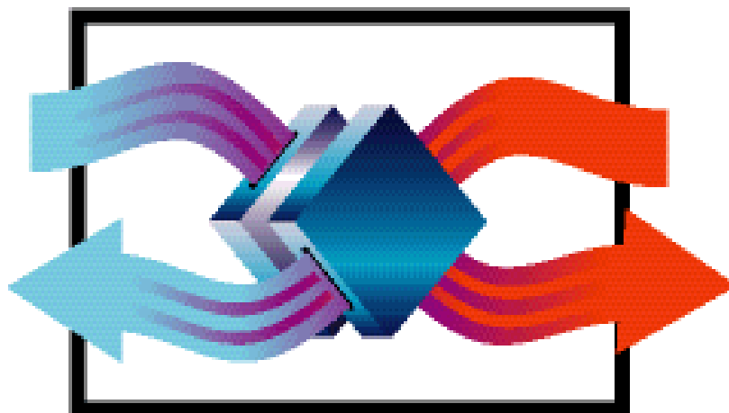
Krossvarmaskiptir (loft / loft).
